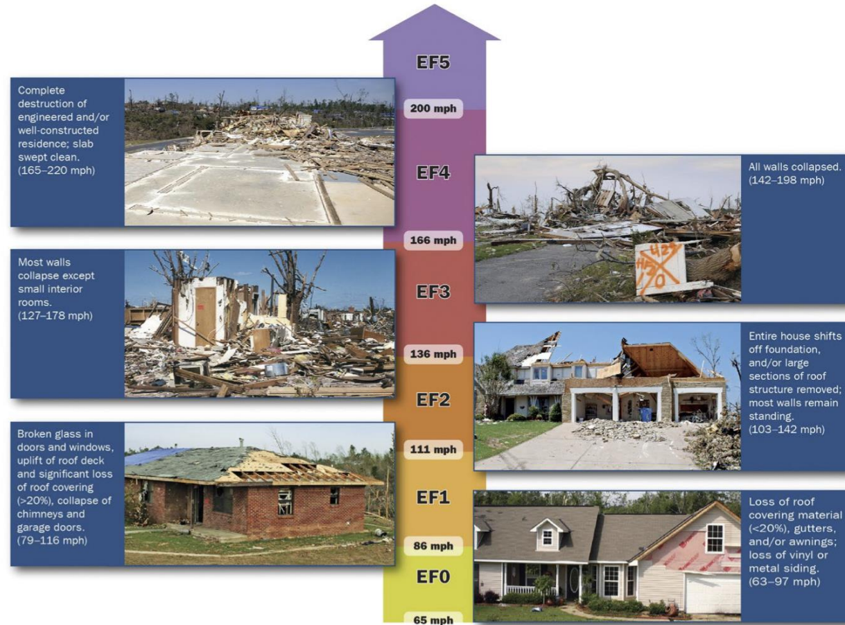
Figure 2-1: Typical tornado damage according to the EF Scale (wind speeds are estimated 3-second-gust wind speeds)
